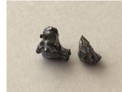
First nugget of Si (99.97% Si) produced during final proof of concept test (About 0.1 g)
